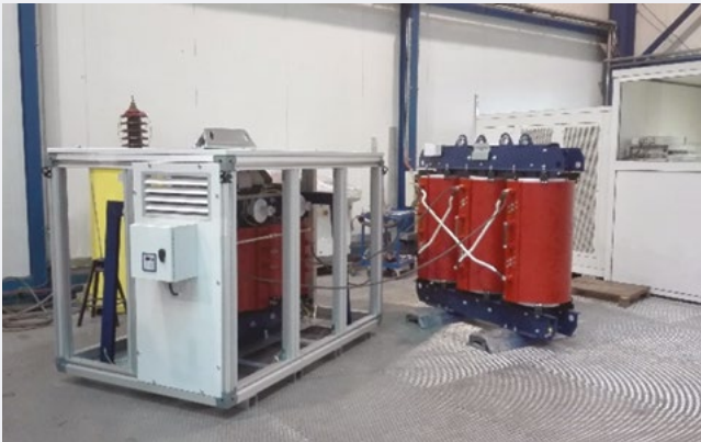
Korndorfer cast resin autotransformer 3018 kVA at 6.6 kV, 50 Hz 11/6.6 kV, insulation class 28 kV, Impulse level 75kVp, overtemperature 85/85°C, Vector group YNa0. Installation on ship board. Destination: UK.
